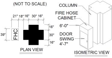
Booth spaces next to a fire hose cabinet (FHC) can have no impediments or obstructions may be placed within 42" clearance area which prohibits the column doors from opening quickly and completely.
